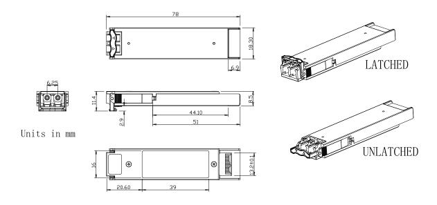
XFP Transceiver (dimensions are in mm)
