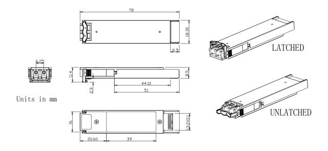
XFP Transceiver (dimensions are in mm)
