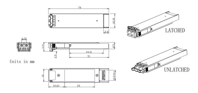
XFP Transceiver (dimensions are in mm)
