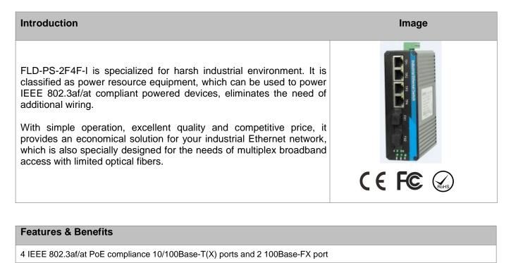
Up to 30W at 48V DC power output on each PoE port
